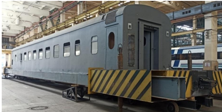
Figure 7. – General view of a prototype dynamometric wagon model 61-907-DM on a stand for loading with longitudinal static loads
