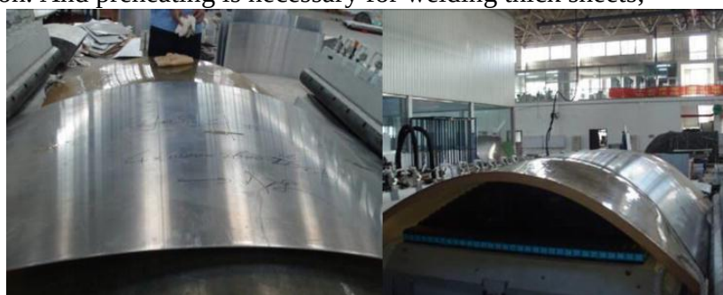
Figure 4. – Sheathing based on a flexible multi-point matrix - Chinese carriage building workshop
