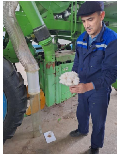
1 – pipe stand to provide air suction, 2 – holder for bundles of raw cotton and small debris, 3 – bundle of raw cotton, 4 – glass pipe, 5 – plastic pipe, 6 – corrugation
