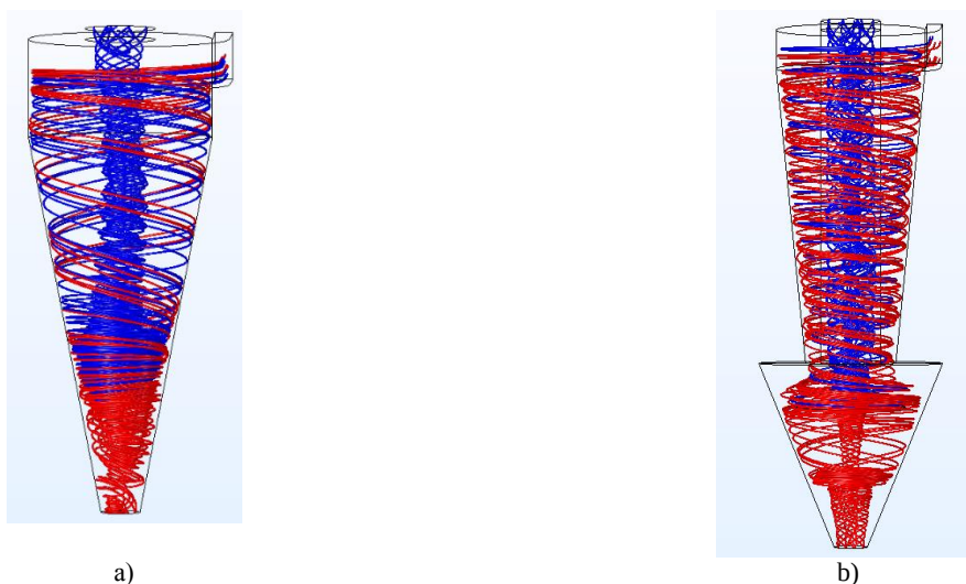
Figure 6- Flow line a) original hydrocyclone, b) recommended hydrocyclone.
