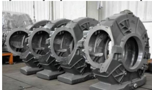
Figure 4. – Typical aluminum gearboxes for CRH series high-speed trains
