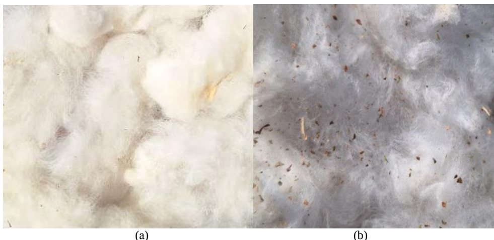
Figure 5. – Raw cotton lobules before testing (a) and after testing saturated with small debris particles (b)
