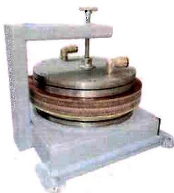
Figure 2. Image of the main module (position #6, Fig.1): A – exterior view; B – sectional view; 1 – heater; 2 – refrigerator; 3 – thermal insulation casing; 4 – test sample; 5 – clamping screw.
